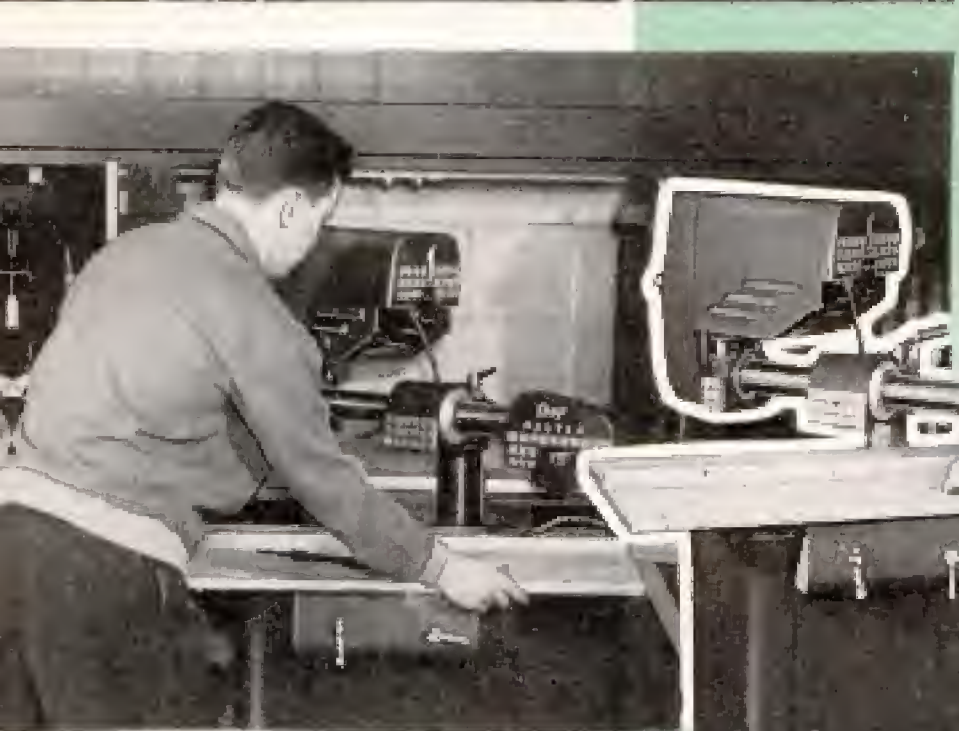
Photo above shows the combination tool being pulled from its niche in the wall cabinet. The two sets of double doors swing wide to provide clearance for the power tool. Photo at right shows tool in use within seconds of its removal from cabinet
